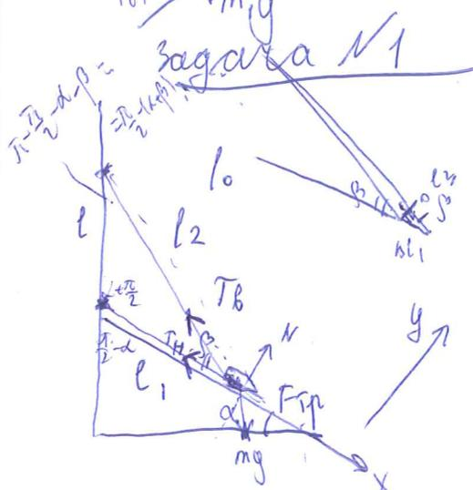
$x: 0 = mg \sin \alpha - T_1 - T_2 \cos \beta + F_{sp} x$
