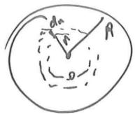
$$J = \int dm \cdot r^2 \quad \left\{ \begin{aligned} J &= \int dm \cdot r^2 = M \cdot r^2 \\ J_k &= M r^2 \end{aligned} \right.$$
